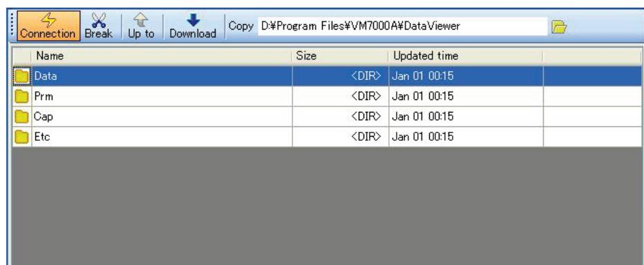
In this case, the file can be downloaded by selecting the "dm file" in the "Data" folder, and pushing "Download".
