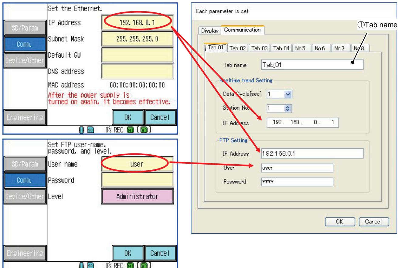
The “IP Address” of “Realtime trend Setting” and “FTP Setting” is set to become it as well as “Paperless Recorder (※Ethernet1)”. (In this case, “IP Address” is set as “192.168.0.1”.)
